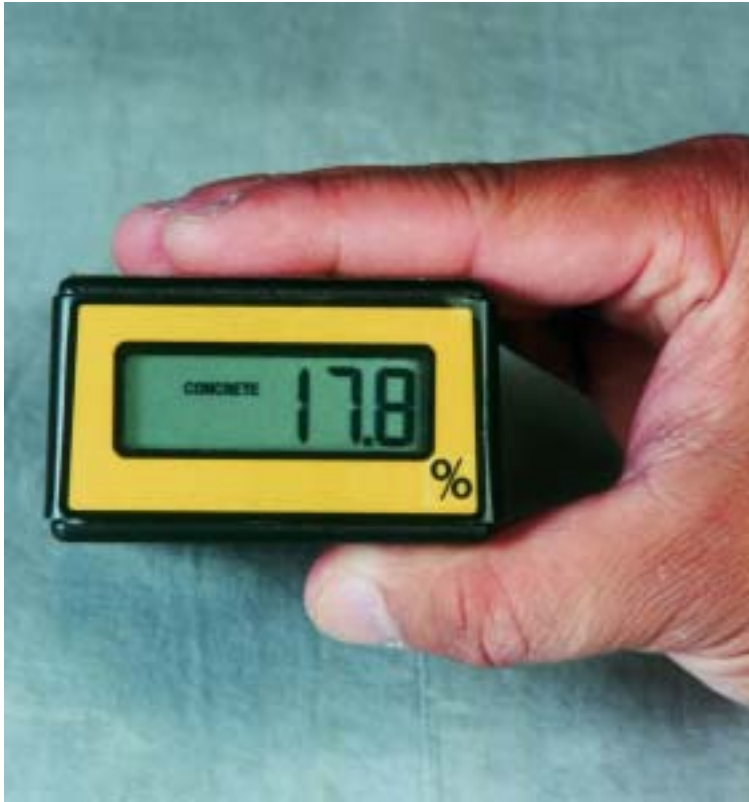
Measuring moisture hidden behind paneling.
